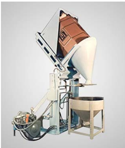
Skip Hoist Hydraulic Dumpers for Discharging the Contents of Any Container
